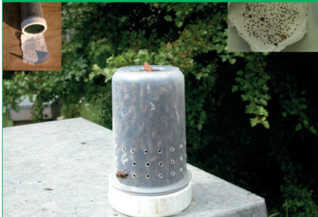
Figure 48: Pyrethroid resistance test kit in use
